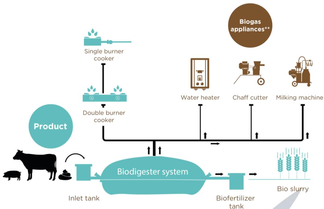
Figure 2: Thermal and mechanical usages with Sistema.bio digesters
