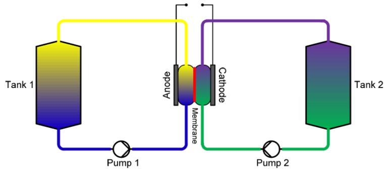
**FigureA.3** – Schematic design of a redox-flow battery [25]
